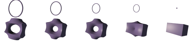
Figure 11: The effect of changing the radius of a circle Voronoi site in combination with the \mathcal{F}_4 operator is shown. This change causes a change of topology by opening and closing a hole in the resulting tiles.
