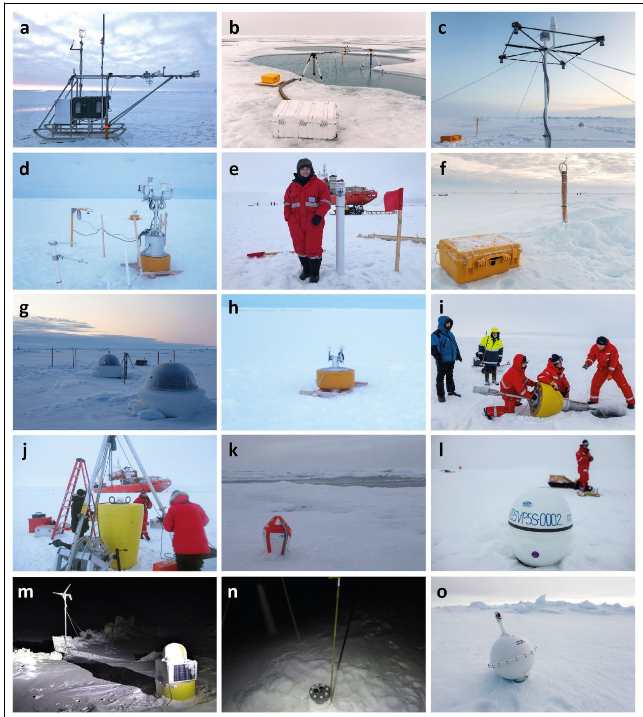
Figure 2. Photographs of selected autonomous platforms (buoys) deployed in the two implementations of the Distributed Network. (a) Atmospheric Surface Flux Station (ASFS #50 at L3; photo by Ola Persson); (b) radiation station 2020R21 and thermistor string buoy 2020T81 deployed on a frozen melt pond (RITBOB; photo by Mario Hoppmann); (c) Snow Buoy 2020S109 (Snow Buoy; photo by Mario Hoppmann); (d) Unmanned (uncrewed) Ice Station (UMIS; photo by unknown); (e) Seasonal Ice Mass Balance buoy (SIMB3; photo by unknown); (f) Snow Ice Mass Balance Apparatus (SIMBA; photo by Mario Hoppmann); (g) Acoustic Zooplankton and Fish Profiler (AZFP) buoy and bio-optical buoy 2020M23 (IMBflex), with ablation stakes in the background (photo by Mario Hoppmann); (h) First Institute of Oceanography Fixed-Level Ocean buoy (FIO FLB; photo by Bing Kong); (i) Drift-Towing Ocean Profiler (D-TOP; photo by Mario Hoppmann); (j) Woods-Hole Ice-Tethered Profiler (WHOI ITP; photo by unknown); (k) position-tracking buoy 2020P162 (ice tracker; photo by Marcel Nicolaus); (l) Salinity Ice Tether buoy (SIT; photo by Mario Hoppmann); (m) Autonomous Ocean Flux Buoy (AOFB; photo by Michael Gallagher); (n) light strings (OptiCAL, formerly Envipope; photo by Dmitry Divine); (o) ice-surface Velocity Profiler 2020P237 (iSVP; photo by Mario Hoppmann). Details of the different platform types are summarized in Tables 1 and S1.
