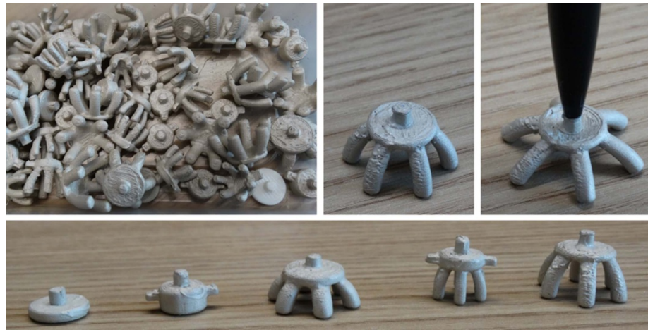
Figure 65. A flexible silver/silver chloride EEG electrode with fingers for passing through the hair. Work reported in [617, 618].
