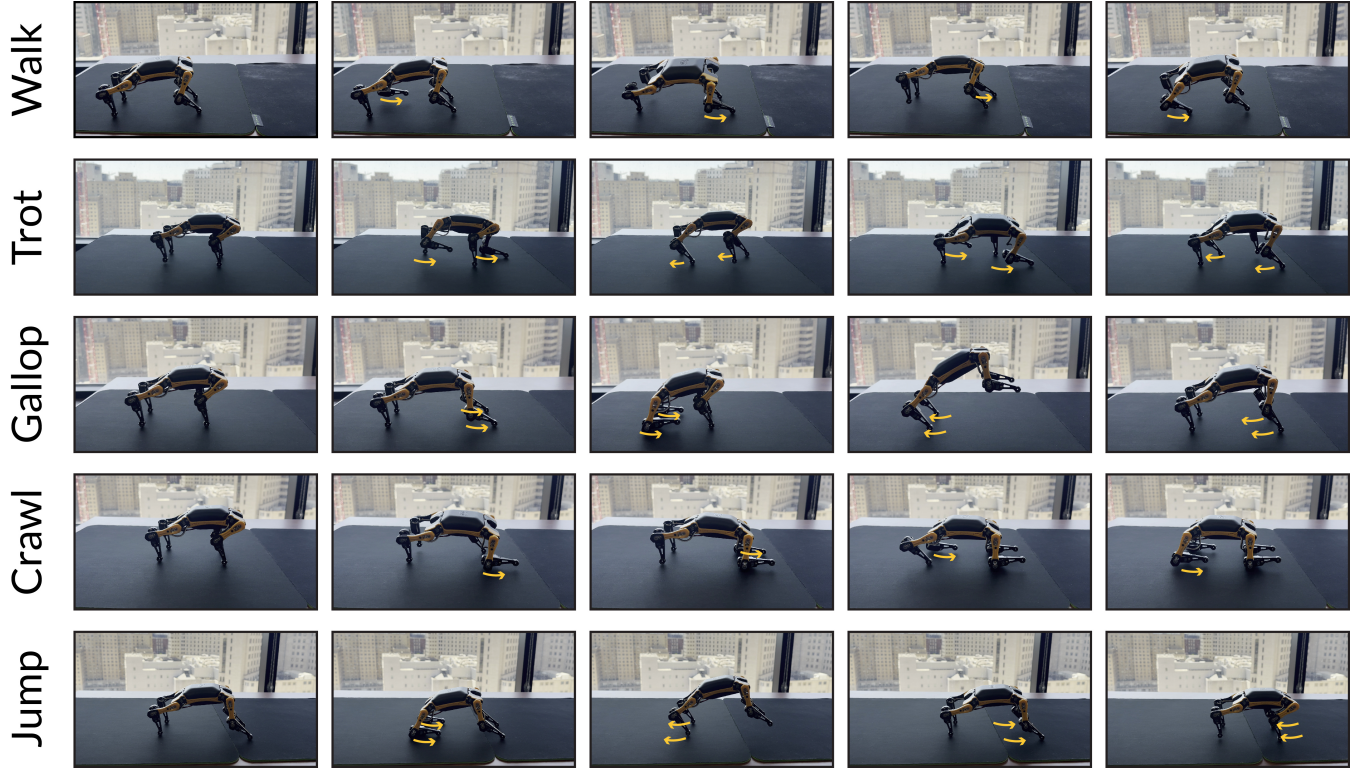
Figure 7. Different modes of locomotion working on the Peto Bittle quadruped. The arrows indicate the motion of the limbs with respect to the previous frame. These photos are snapshots of the robot actually executing the gait patterns. Demo video can be found at https://youtu.be/9AKoM28ix68
