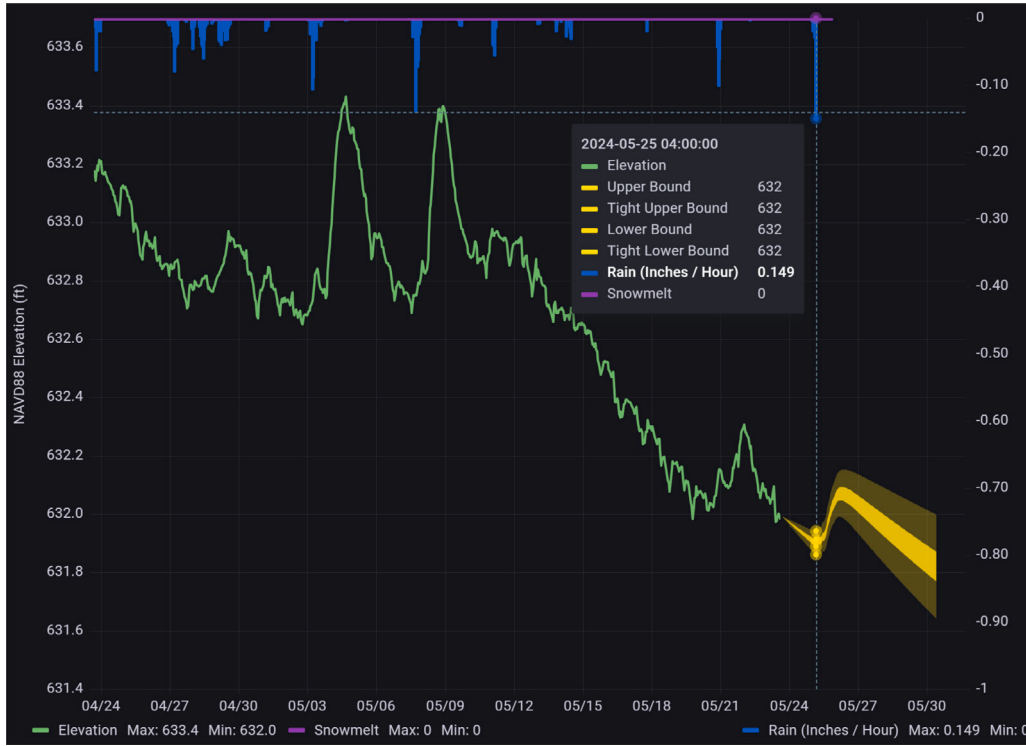
Fig. 2. Sample decision support dashboard. Estimated snowmelt and rainfall (across all flow-distance regions) are indicated on top of the graph in purple and blue respectively. Historical water surface elevation is in green. Predictions with uncertainty estimates are provided in yellow.
