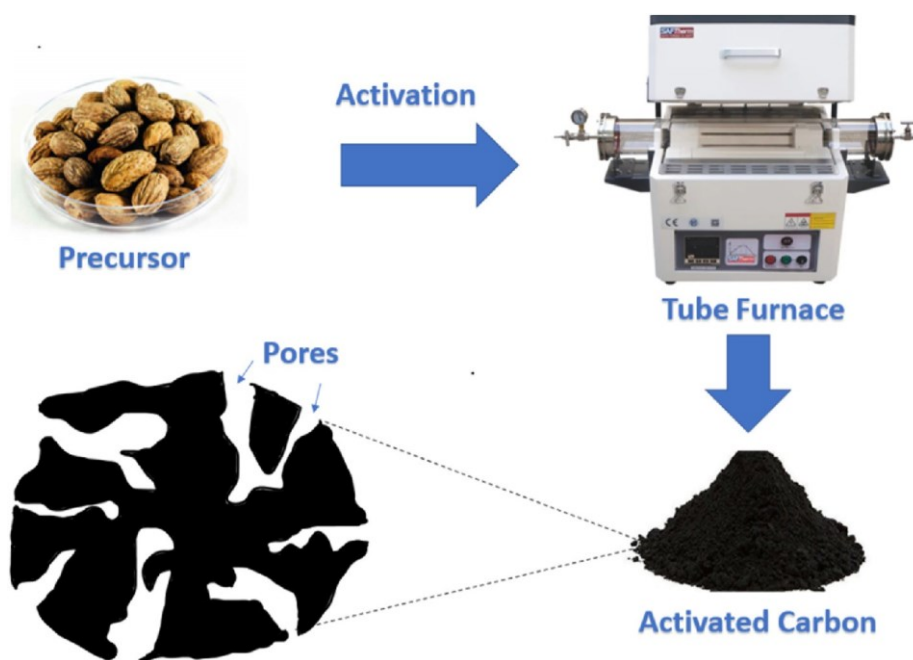
Scheme 2. Activated carbon processes from biomass precursor.
