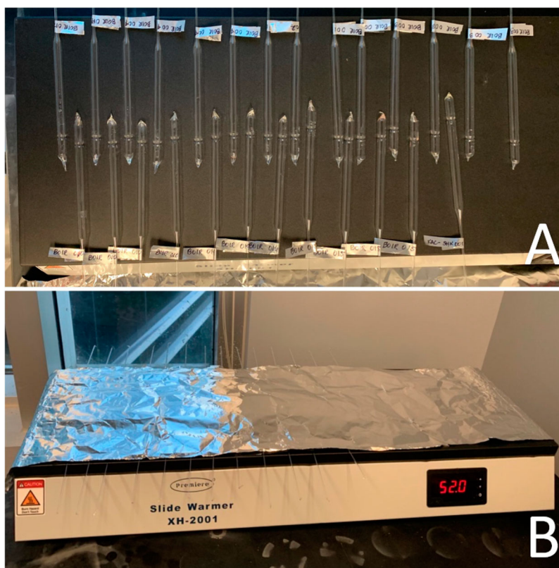
Figure 6. A. Slide warmer with pipettes positioned so the narrow end is slightly hanging off the side while the larger end is positioned within the heated area to allow condensation to occur. Each pipette is labeled and wrapped with aluminum foil for easy identification later. B. An aluminum foil cover can be placed over the slide warmer after all pipettes are positioned to help trap heat and allow for proper condensation of sample from the larger end to the narrow end.
