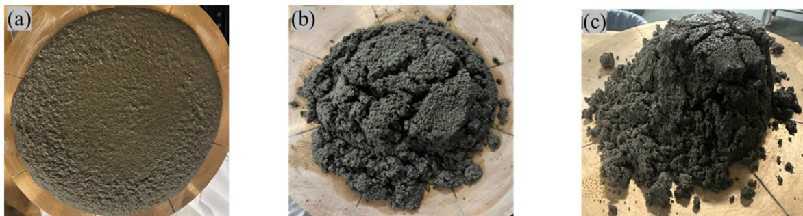
Fig. 2. Flow diameter measurements of mortar samples containing (a) 0% CNF, (b) 0.05% CNF, and (c) 0.3% CNF.
