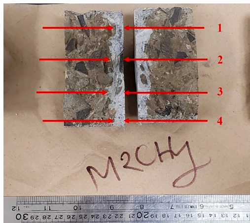
Fig. 4. Measurements of chloride penetration depth.
