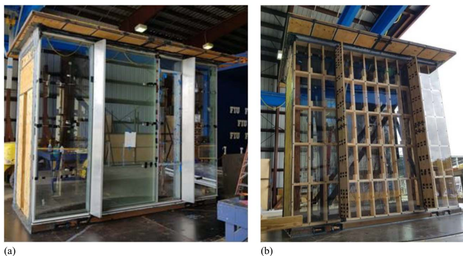
Fig. 3. Curtain wall with vertical protrusion: (a) glass curtain-wall panels; and (b) polycarbonate panels.
