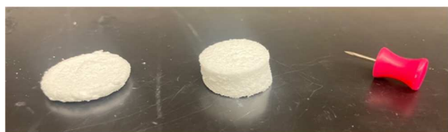
Figure 2. Image showing the appearance of (left to right) fixed polyMIPE, recovered polyMIPE, and thumbtack for size reference.
