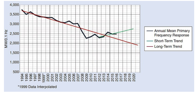
Fig. 2. Decreasing trend of IFRO from the eastern interconnection according to NERC report 2017 [4].
