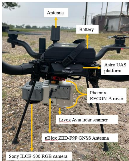
Figure 2 A typical setup before a flight showing the RECON-A payload and the Astro UAS platform.
