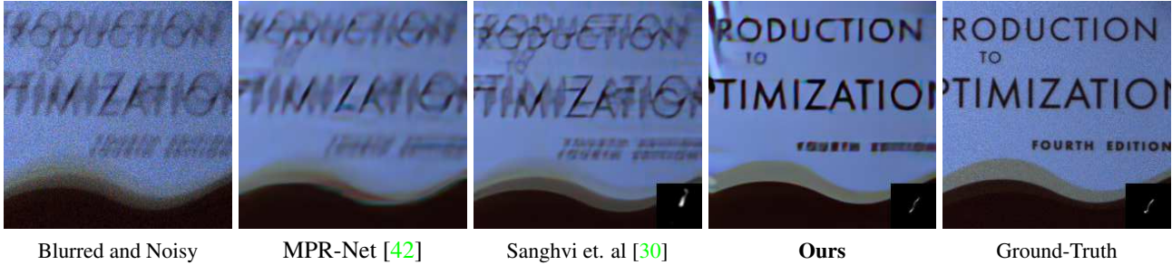
Figure 1. The proposed Kernel Trajectory Network (KTN) on real noisy blurred image from Photon-Limited Deblurring Dataset (PLDD) [29] The result corresponding to MPR-Net was generated by retraining the network with GoPro dataset [24] corrupted by Poisson noise. The inset images for "Sanghvi et. al" and "Ours" represent the estimated kernel and the inset image for "Ground-Truth" represents the kernel captured using a point source, as provided in PLDD.
