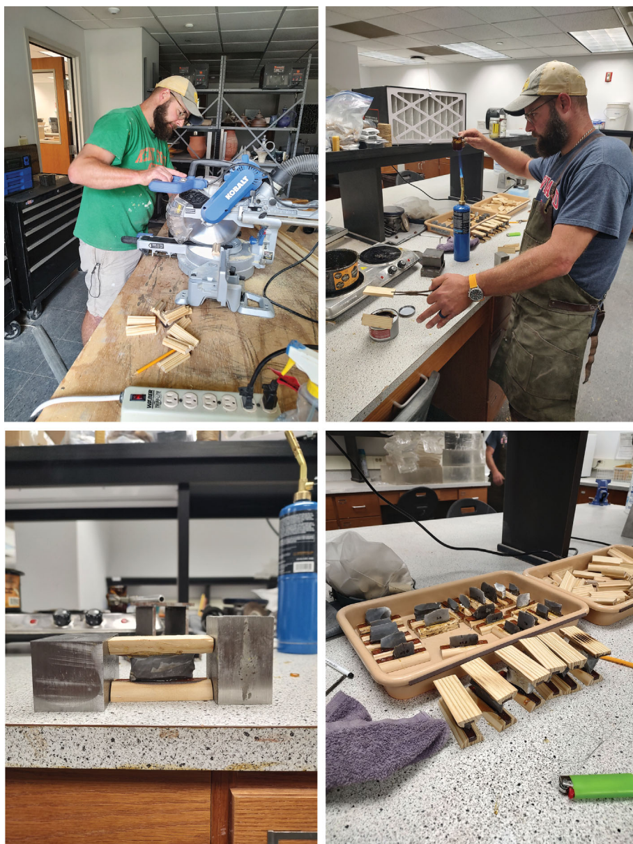
FIGURE 2 Procedure for creating the test specimens started with cutting pine wood and giving each piece a standardized 'trough' (top left). Test specimen components were heated (top right) and then hafted together (bottom left). All the backed edges were hafted first, then the sharp edges (bottom right). See the main text for details.
