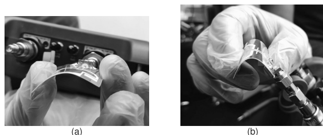
FIGURE 17. Images of fabricated antenna bending. (a) Horizontal bending, (b) Vertical bending.
