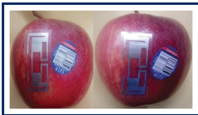
Fig 6. Fabricated prototype of RFID tag on two different apple samples. 111
