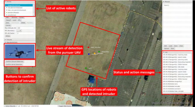
Fig. 2: Graphical user interface for multi-robot cooperative C-UAS operation.
