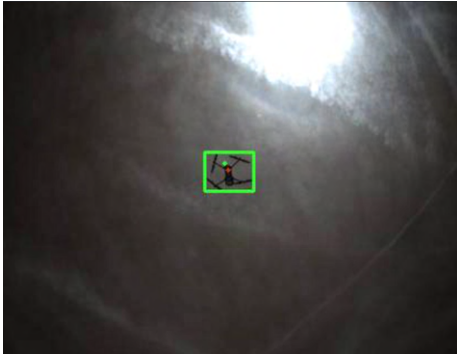
Fig. 9: Image detection of DJI Mavic Pro. The output of the detection module is depicted in green with a bounding box and the dot representing the intruder's position estimated by the radars. The red dot is the combined estimate after being filtered by the extended Kalman filter.
