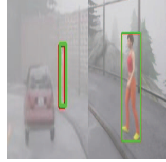
Fig. 4: Objects detection by YOLOv8 to locate the pedestrian. Left: ego vehicle's view, Right: helper vehicle's view. The green box is the ground truth and the red box is the predicted bounding box by YOLOv8.
