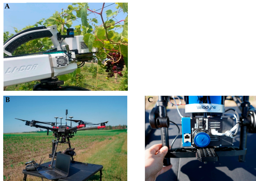
Figure 1. (A) Fully developed, sun-exposed leaves measured by LiCOR 6800 as ground-truth or directly measured variables. (B) UAV platform (DJI Matrice 600 drone) for indirect measurement of physiological traits through aerial remote sensing. (C) Nano hyperspectral headwall sensor fixated in gimbal carried by UAV.
