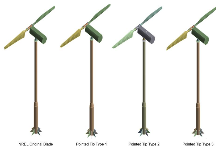
Figure 7. Numerical model of NREL Phase VI wind turbine with different tips.
