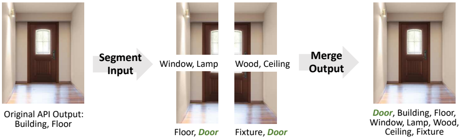
Fig. 13. Tackling focus mismatch with segmentation in RoomR (Figure 6).
