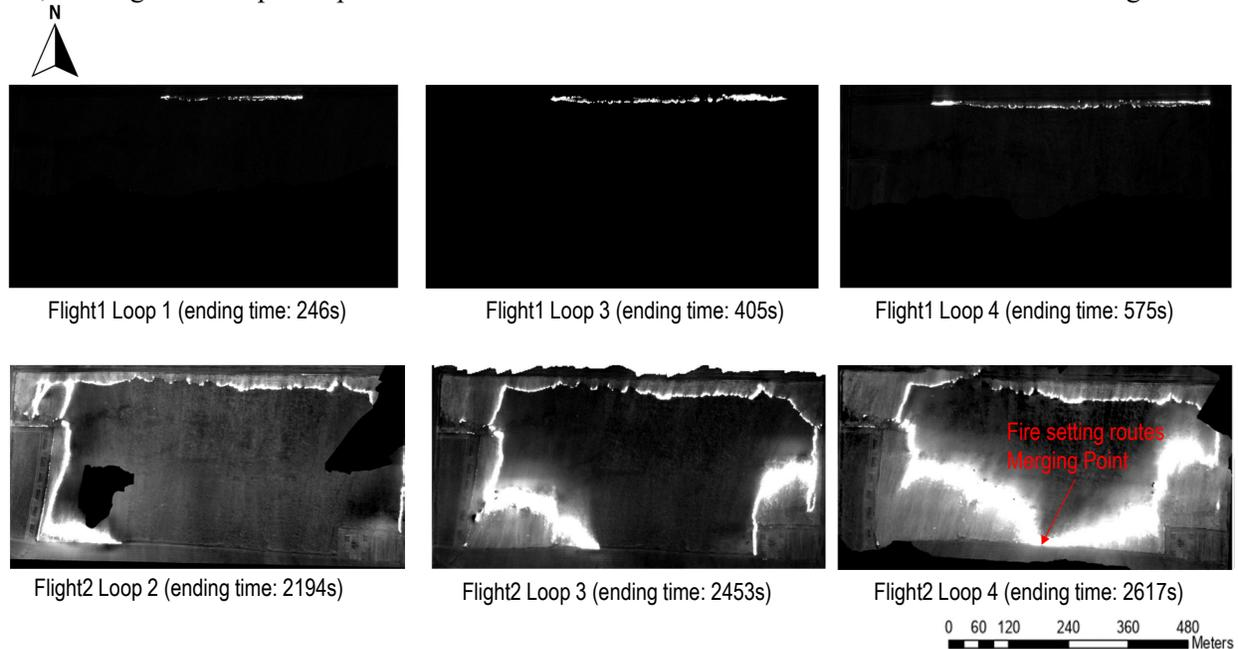
Figure 3: Thermal maps of the prescribed fire from Flight1 and Flight2 (white color represents the burning fire front of the prescribed fire)
