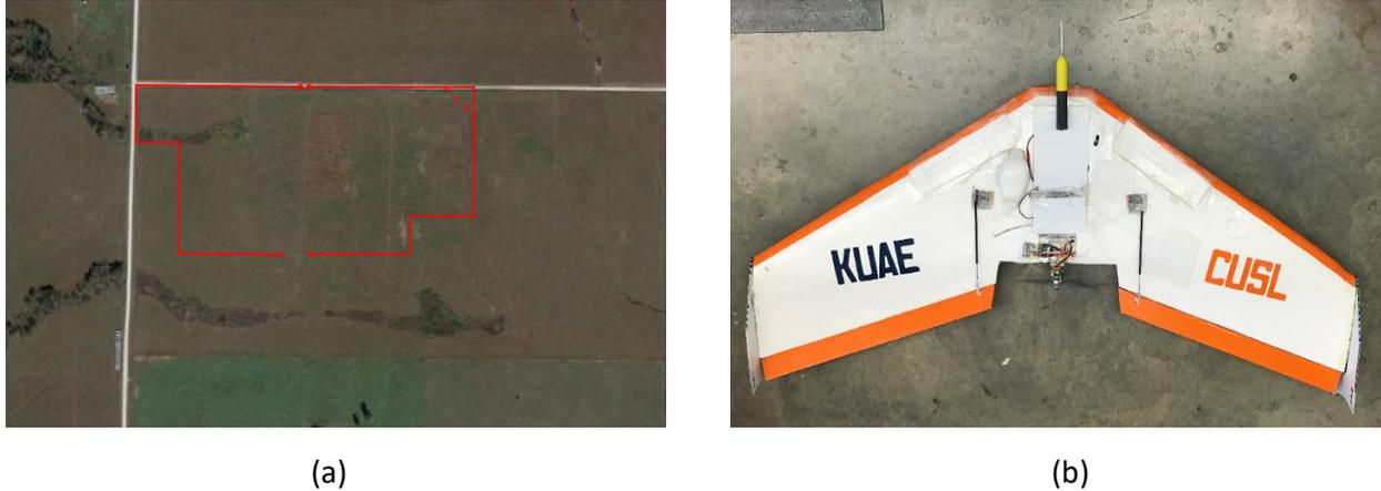
Figure 2. Prescribed Fire Area and the KHawk UAS: (a) Prescribed fire area and fire setting routes (illustrated by the red lines in figure); (b) KHawk Zephyr 55 Thermal UAS.
