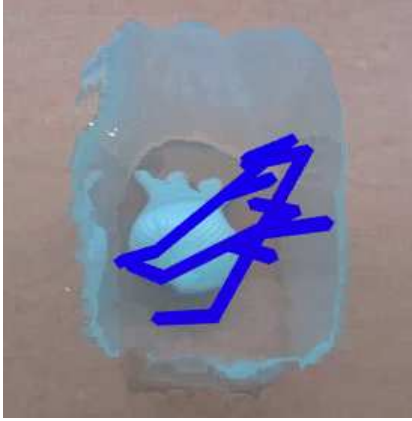
Fig. 3. Output of DFNet by Fang et al [8] on one of the translucent container test objects.
