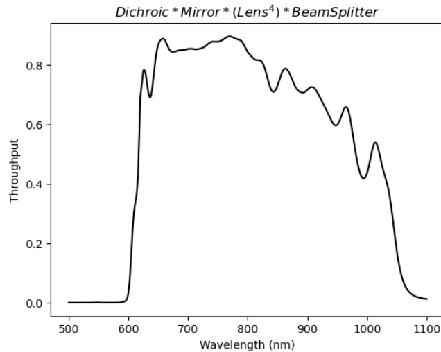
Figure 4. Combined optics throughput (Dichroic, Mirror, Lens, and Beam Splitter).
