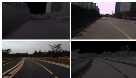
Figure 1. Left: Input thermal (first row) and color visible (second row) images. Right: Our cross-domain image translation result to color (first row) and thermal (second row) domains. Our CCGAN network is able to recover more details and keep scene boundaries clear with the proposed constraints.
