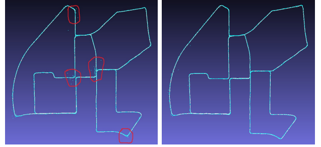
Fig. 5: Vehicle paths generated without dynamic online training range determination function (left) and with this function (right). Red color marks the region of major difference.
