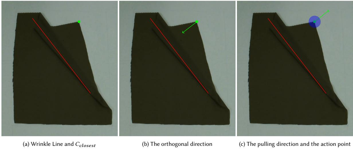
Fig. 6. (a)  $C_{closest}$  is determined by the two-step minimization process, (b) The orthogonal direction is determined which is pointing towards the wrinkle, (c) The direction is fixed using the position of the intersection  $I$ .
