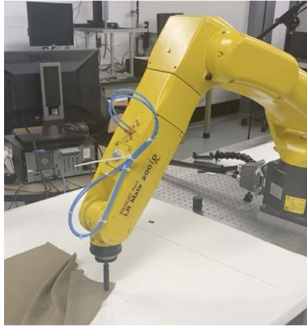
Fig. 1. Fanuc LR/Mate robot arm manipulating fabric
