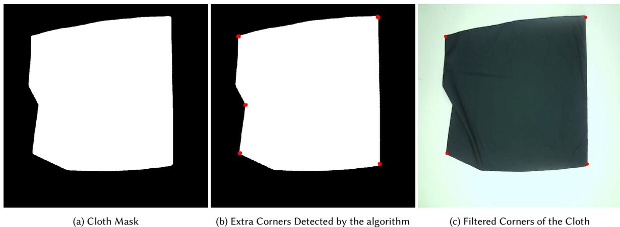
Fig. 5. (a) Initially, the cloth mask is identified using a deep learning method, (b) followed by the detection of corners using the Harris Corner Detector, (c) and then the four corners are pinpointed by calculating the shortest distances from the four corners of the frame.
