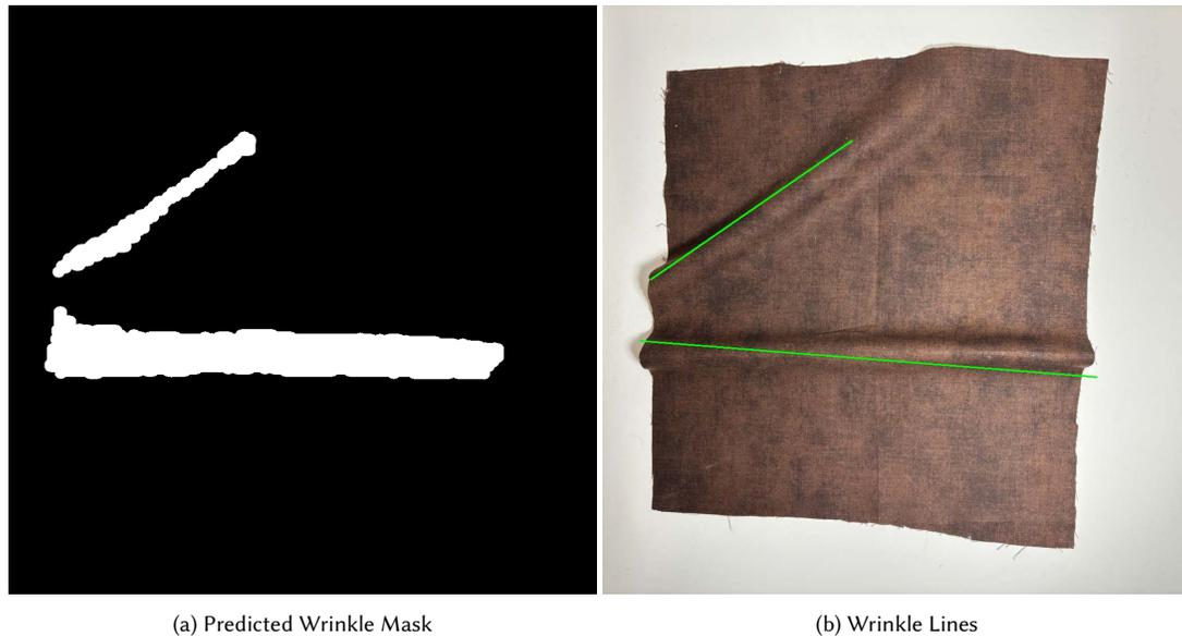
Fig. 4. (a) Initially, the wrinkle mask is identified using a deep learning technique and (b) subsequently, lines that align with the wrinkles are determined through computer vision algorithms.
