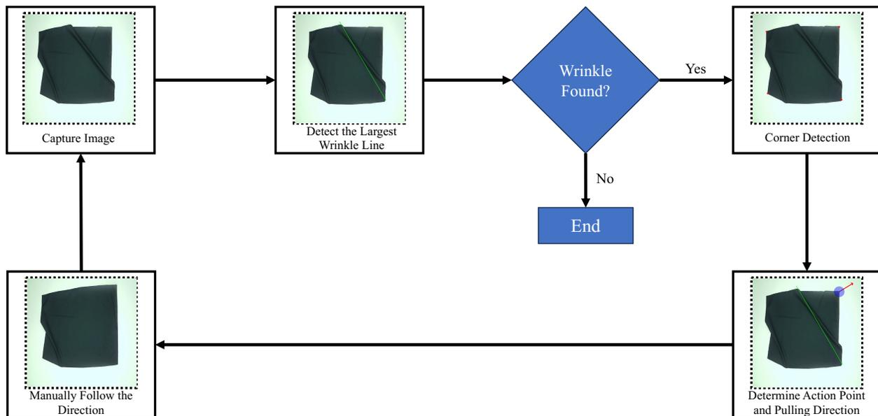
Fig. 2. The overall workflow of our proposed method to flatten a cloth
