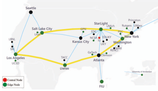
Fig. 6. In our experimental deployment utilizing FABRIC [12], covering 17 sites in the USA and Europe, Indiana University hosted the central node, and each site accommodated 2 edge nodes.
