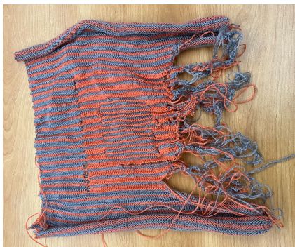
Fig. 21. An attempted illusion knit without path planning. Note that the failure manifests not as mere visual artifacts on the knit object, but in the fact that the knit is structurally not a surface at all on the right side, and nothing is viewable.
