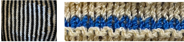
(a) A top-down look at a single-view pattern. The knitted version is depicted in Figure 4b. (b) A close up of the microgeometry of single-view patterns. At the bottom is a row of yellow purl bumps, below blue and yellow knits. The yellow purl bumps are raised above the fabric.
