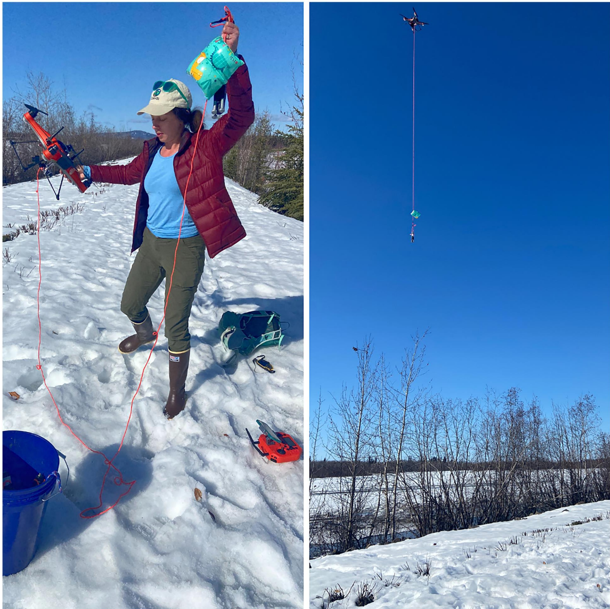
Figure 8. Left: SILT scientist J. Davis untangles the line connecting the drone to the turbidity sensor to prepare for the next test flight with the water wing flotation device prominently displayed. Right: The drone in flight with the water wing flotation device clearly visible.
