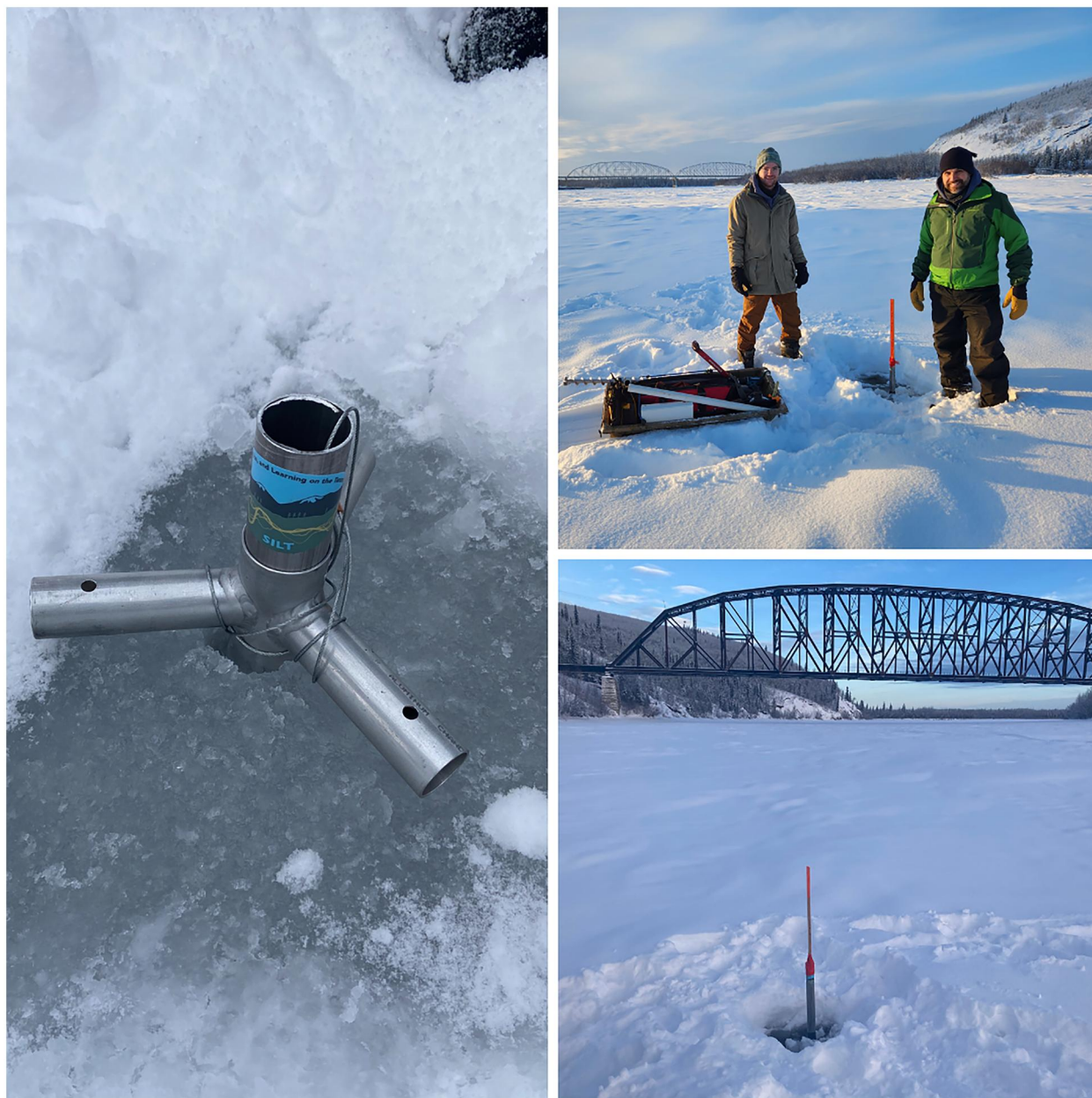
Figure 5. The turbidity sensors were housed in metal pipes (left) and fitted with bright orange stakes for visibility and safety on the Tanana River (top and bottom right).
