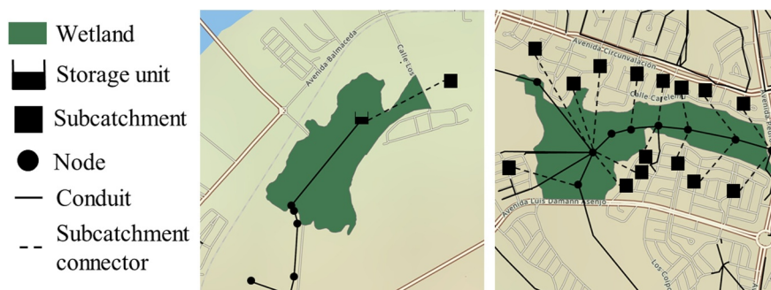
Figure 4. Example wetlands in Valdivia illustrating differences in the construction of storage unit and conduit wetlands in EPA SWMM. The wetland on the left receives water from a single subcatchment and was modeled as a storage unit. The wetland on the right receives water from multiple subcatchments and was modeled as a series of conduits and nodes.
