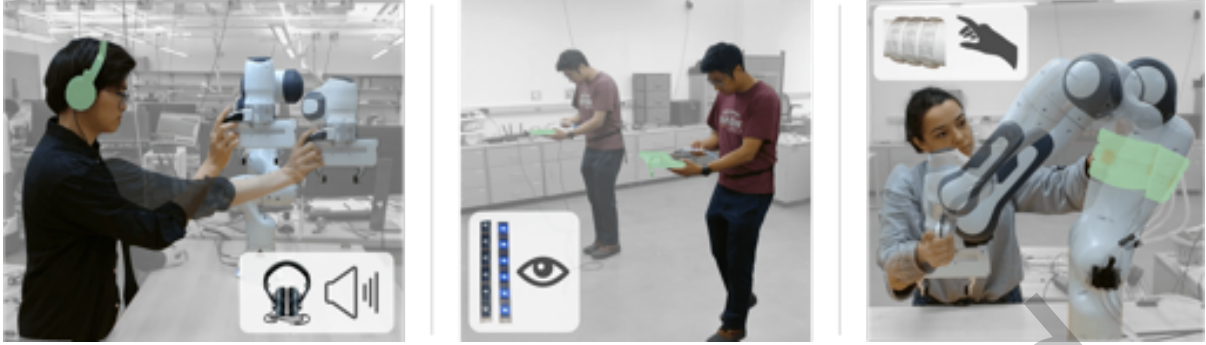
Fig. 8. Interfaces and tasks for our in-person study. (Left) In Sounds the human moved a robot arm back and forth along a single axis. The interface played a musical note of varying pitches to convey the correct arm position. (Middle) In Lights participants walked around an empty space. The interface illuminated two LED strips to indicate the location of their missing phone. (Right) in Haptics we wrapped pneumatic bags around a robot arm [38]. Participants needed to guide the robot to the correct height, orientation, and distance from their body: the interface inflated and deflated the haptic bags to convey these features.
