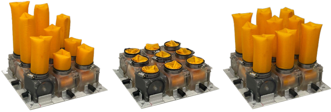
Fig. 7. (Left) A diagonal slant surface can be transitioned to (Right) a flat, planar inflated surface. However, given the hysteresis in the retraction mechanism, the surface must transition first through the rest, deflated state (Center).
