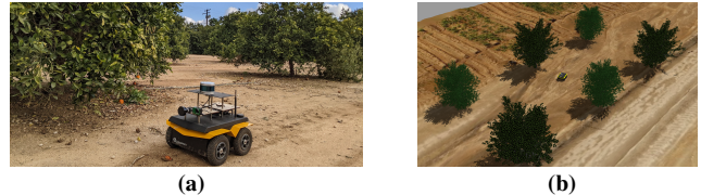
Fig. 1: (a) Clearpath Jackal equipped with a Velodyne VLP-16 LiDAR and a MAPIR Survey3N RGN camera during field experiments. (b) The designed simulation world in Gazebo along with the simulated Jackal mobile robot. This world model contains a 2 \times 3 tree grid of 3 orange and 3 lemon trees placed at a 5\text{ m} width \times 5\text{ m} length relative distance from each other.
