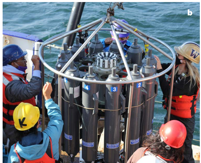
FIGURE 1. Geoscience Education, Oceanographic Discovery, Undergraduate Collaboration (GEODUC) program participants engaged in geoscience research during the summer bridge program at Friday Harbor Laboratories (a) build a temperature sensor for deployment, and (b) ready a CTD with Niskin bottles for deployment.
