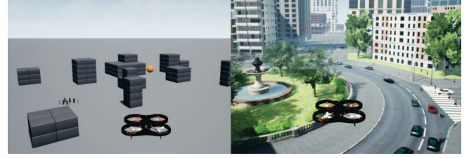
Fig. 3. Two maps from Microsoft AirSim: on the left is "Blocks" which contains static objects with arbitrary shapes and sizes, and on the right is "City" which contains both static and dynamic objects expected to be encountered in the real world.
