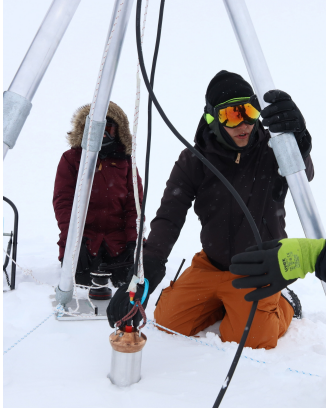
Figure 2: Melting probe in operation during the 2023 RNO-G field season.
