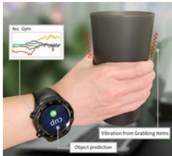
Fig. 1. ViObject is a system that recognizes untagged everyday objects using accelerometer and gyroscope sensor data from commodity smartwatches. Passive object recognition is accomplished by identifying the vibrations caused by grab-objects without the need for additional hardware or human effort.
