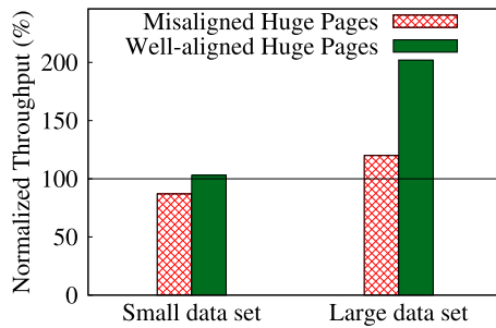
Fig. 7. Well-aligned huge pages can effectively reduce address translation overhead. Throughput is normalized to that of vanilla Linux/KVM.
