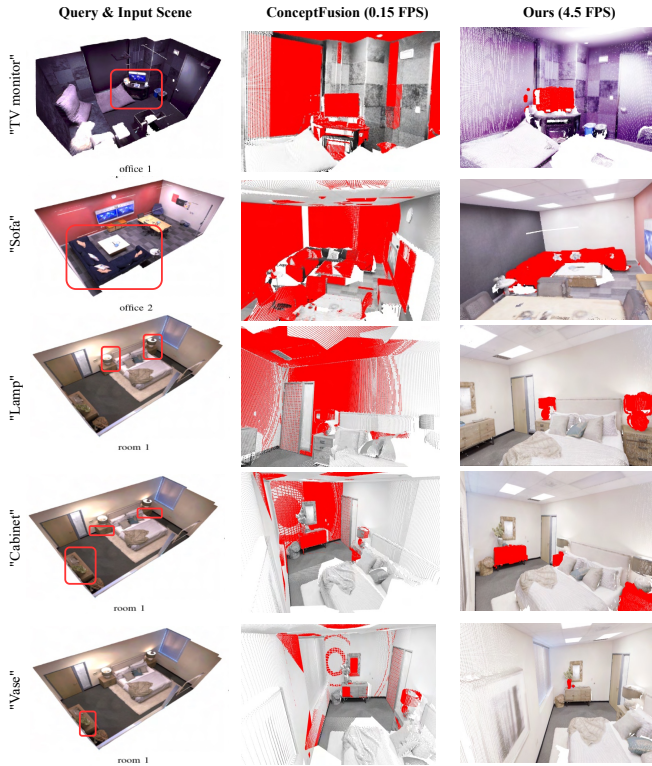
Fig. 2. Qualitative comparison of 3D object query results on Replica dataset. While ConceptFusion failed to pinpoint the object location, Open-Fusion can estimate more precise location from language queries.
