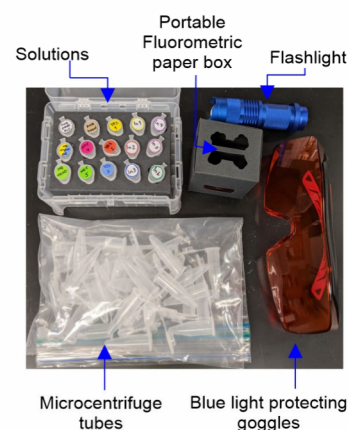
Figure 4. Setting up the materials and reagents. (A) Arrangement of 15 different microcentrifuge tubes (represented by circles) filled with solutions needed for constructing and testing the three DNA logic circuits: one tube with DNA grade water (black), one tube containing the assembled DNA board (brown), three tubes with different YES gates (orange), two tubes with different NOT gates (blue), two tubes with the MB probe solutions to report the output of the IMPLY/OR circuit and NAND circuit (purple), and six tubes containing individual inputs (green). (B) A tube-holder box made of black cardstock paper for holding samples containing four different input combinations of one DNA logic circuit. The samples are irradiated with a blue LED flashlight for output visualization at a 90° angle. (C) All necessary materials and reagents can be conveniently packaged into a 19 × 16 × 8 cm box as a portable education kit for the DNA molecular computing activity.
