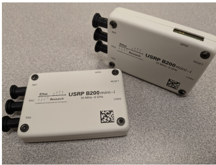
Fig. 4: Ettus USRP B200 used for collecting OTA dataset.
