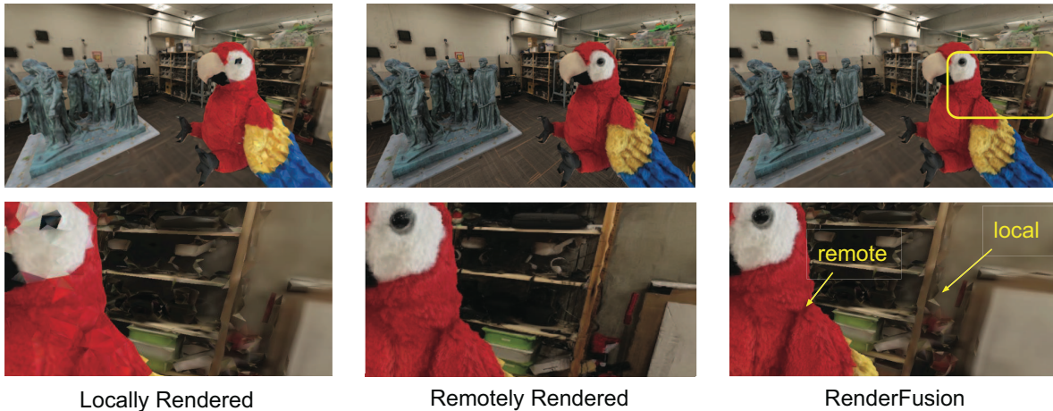
Figure 1: Rendering quality of local and remote rendering compared to RenderFusion. In this particular scene and viewport, RenderFusion selects the high-complexity background object to be locally rendered at a lower resolution and the statue and parrot models to be rendered remotely at a high resolution.
