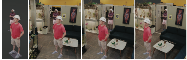
Figure 11: A qualitative result of two high-resolution people reconstructed in 3D from our testbed (using 4 RGB-D cameras), composited with a photogrammetry background, and rendered from three arbitrary viewpoints.
