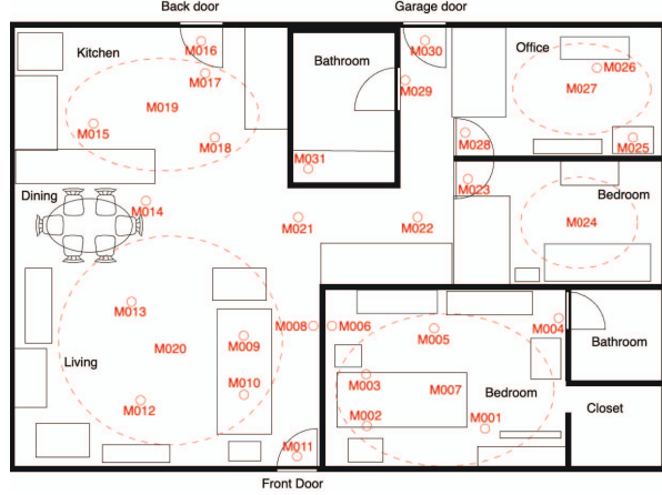
Figure 2. Location of motion sensors in smart home. The dotted ellipses with text in the center represent infrared motion sensors with a wide area of detection. The other sensors, represented by small circles with text above or below, are sensitive to motion in a one meter circle directly below the sensor.
