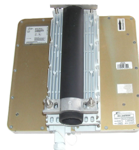
Fig. 17. Alvarion transceiver with massive heat sink fins.
