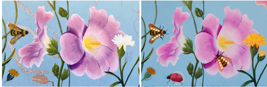
Fig. 2. Detail from an interactive mural that uses copper tape and CuPro-Cote. Left: During construction circuits are made with copper tape and touch sensors are painted with CuPro-Cote. Electrical connections between materials are made by painting conductive paint over copper tape. Right: The circuitry and touch sensor have been painted over with non-conductive paint. Touching the lady bug activates different light patterns. This mural is 32 feet wide by 10 feet tall ( 10 \times 3 m).
