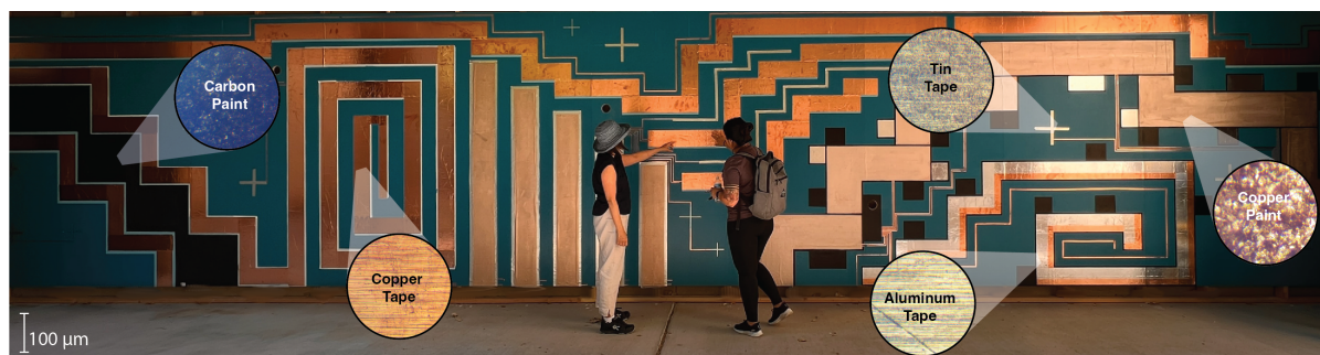
Fig. 1. An Interactive Mural that uses conductive paints and tapes for both functional and aesthetic purposes. Materials are used as capacitive touch sensors as well as visual design elements. This 44 \times 10 foot ( 13.5 \times 3 m) mural is permanently installed outdoors. The scale in the lower left hand corner applies to all microscopic images of materials, shown in circles.
