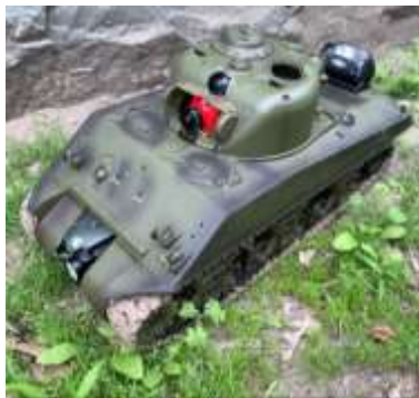
Figure 3 Mobile inspection robots: a. HIVE 2.0 culvert inspection robot [5], and b. Water sampling UAV robot under development for modification to inspect the underside of bridge decks.
