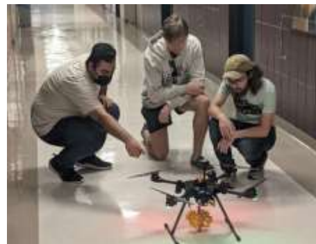
Figure 3 Mobile inspection robots: a. HIVE 2.0 culvert inspection robot [5], and b. Water sampling UAV robot under development for modification to inspect the underside of bridge decks.
