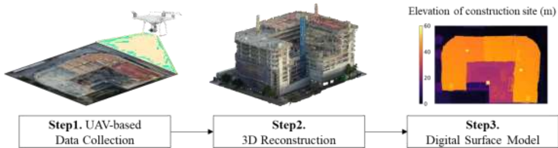
Figure 2. Procedures for site geometry data acquisition.
